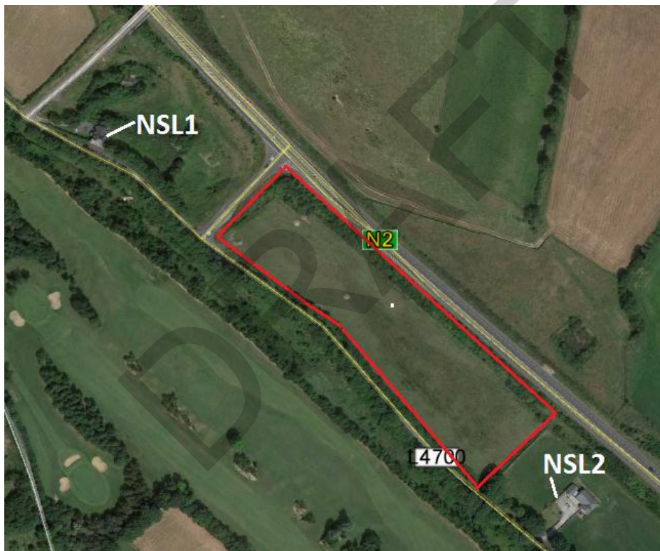
Figure 9.1: Construction Compound Noise Monitoring Locations
